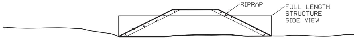
ROUND PIPE FULL SLOPE LENGTH, NO WINGWALL (Cross Section View)
