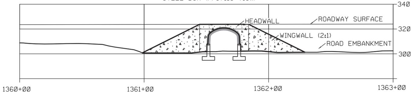
PRECAST CONCRETE SPAN (Profile View)
